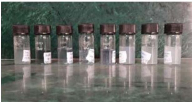
Figure 3: Bottle test experiment for gel strength and gelation time
